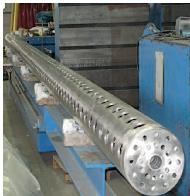
Acceptance of immersion heaters on the PHÉNIX installation
