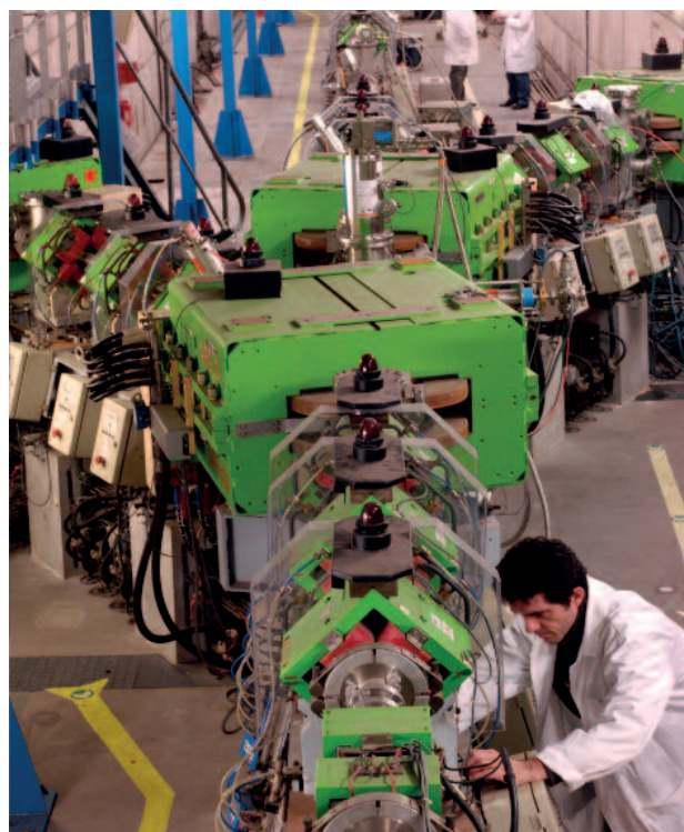
The "fishbone" in the GANIL, which guides the beams in the experiment halls
